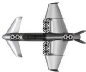
Four of the latter are set vertically in the fuselage (two aligned in the nose and two behind the power unit, which is installed just past the crew compartment, over the wing). These thrusters are used for vertical take off and landing and are closed by panels in cruise.
