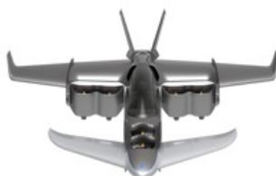
The other four thrusters are installed at the wing roots, mounted on paired tilting units, to contribute for vectored thrust in V/STOL operations and for transition to/from horizontal flight. They are set in horizontal for fast cruise propulsion.
